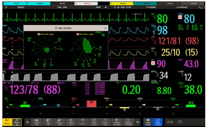
ST Map gives clinicians an integrated view of directional ST movements, allowing for a shorter reaction time than traditional ST indexes, saving crucial minutes.
